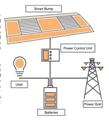
This linear generator uses the electromagnetic induction principle to transform the movement into power. The power produced is carried out into a circuit where the voltage is leveled, steadied and regulated.
